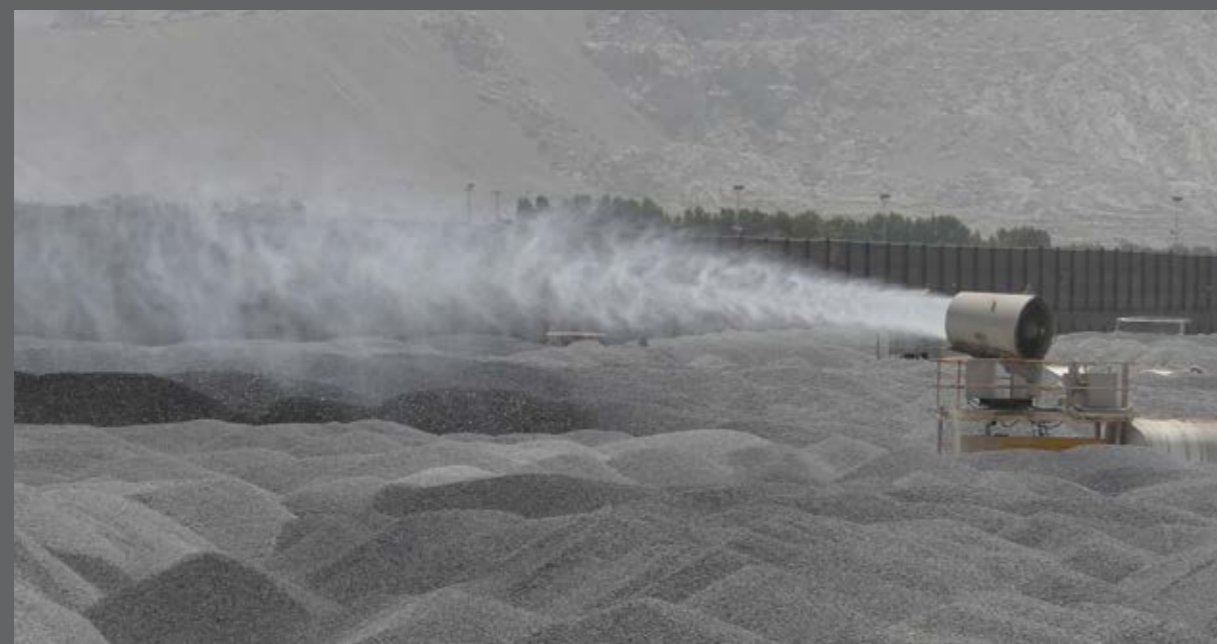
SPRAYING WATER MIST ONTO AGGREGATE STOCKPILES AT STEVIN ROCK HARBOR
